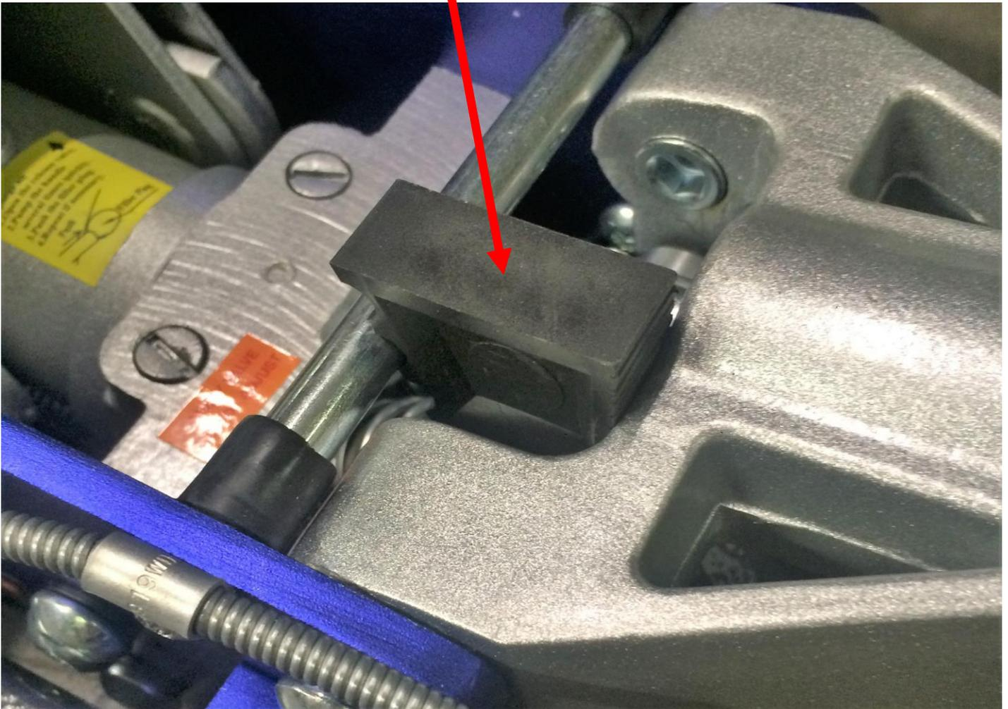
Insert round jack handle into mechanism and push down firmly. Remove plastic insert.
