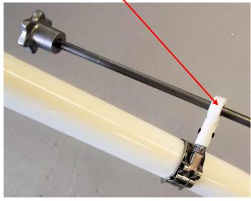
(3) Insert locking knob upper shaft into lower shaft connector noting that machined flat aligns with set screws. Tighten set screws securely.
