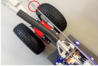
(4) Tighten locking knob CW after helicopter tow pin engaged and helicopter skids raised +/- 2" above surface.
