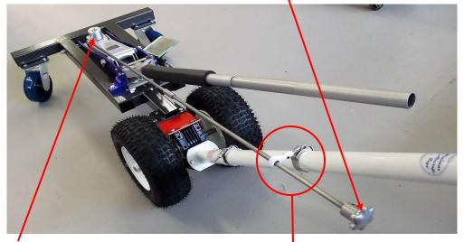
(5) Lower helicopter onto skids allowing lifting head to retract completely.
