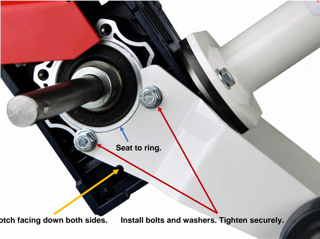
Notch facing down both sides. Install bolts and washers. Tighten securely.
