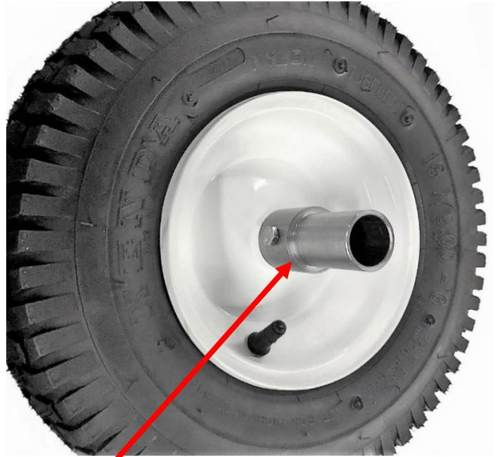
Install weight hub onto wheel. (May require tapping with a rubber mallet or wood block with hammer.) Align hub bolt holes with wheel bolt holes. Align holes with axle hole. Install 1/4" x 2" bolt and lock nut. Tighten securely.
